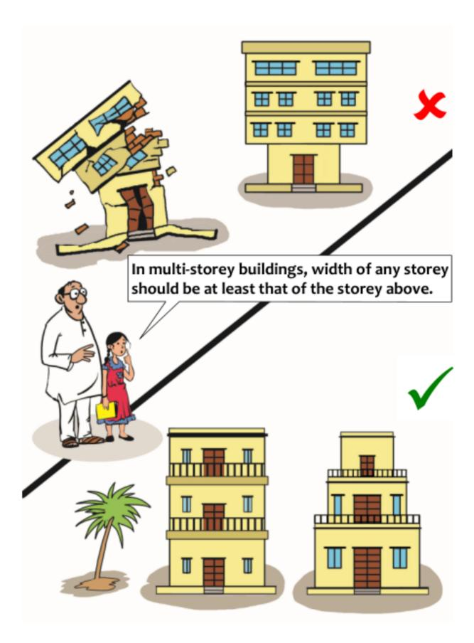
Shape of a Building in Elevation
