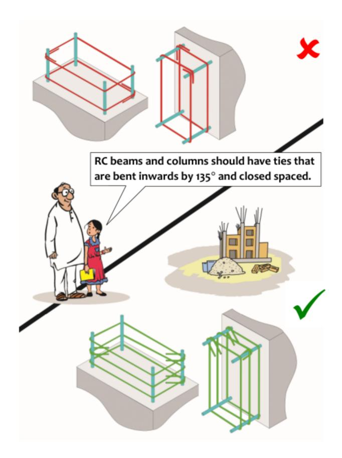
Providing 135° Hooks in Steel Ties
